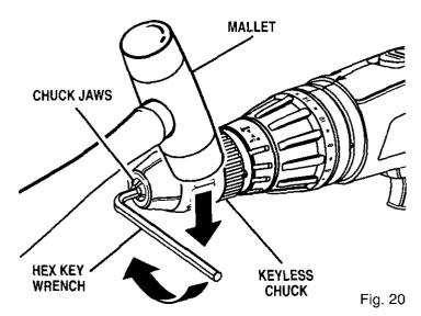
Open chuck jaws and remove wrench. Remove the chuck screw by turning it in a clockwise direction. See Figure 21.
